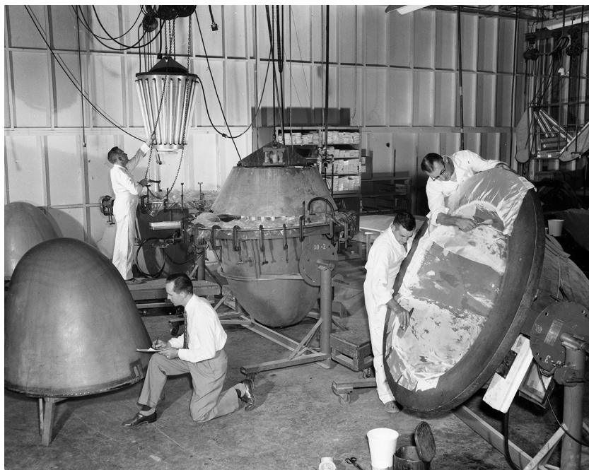
Workers molding bomber blisters at the Goodyear Aircraft Corporation's Litchfield Park facility. Arizona Historical Society–Tucson collections, MS1255, Charles and Lucile Herbert–Western Ways Features Manuscript and Photographic Collection, Box 28, Folder 420.
