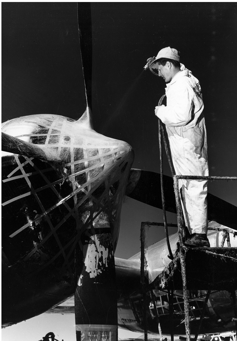
Worker de-cocooning an airplane. Arizona Historical Society–Tucson collections, MS1255, Charles and Lucile Herbert–Western Ways Features Manuscript and Photographic Collection, Box 35, Folder 536.
